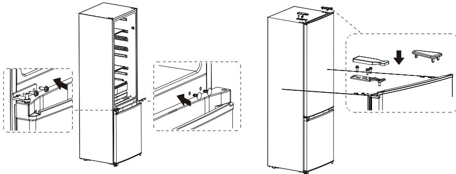
The following must be confirmed before installing the top hinge cover. The screws that hold the hinge should be tightly pressed against the hinge surface to ensure that the screw is not deflected. After the hinge is installed, make sure there is no shaking.
