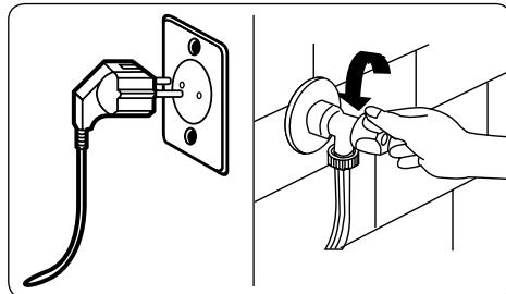
Before any maintenance or cleaning operation, switch off the mains power supply and unplug the machine. Turn off the water supply before starting any maintenance or cleaning.
