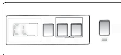
If one of the buttons is pressed or if the selected program is changed using the program selector while the child lock function is activated, the "CL" symbol starts flashing on the electronic display for 2 seconds.
