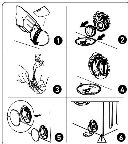
The washing machine's drain pump filter system prolongs the lifetime of the pump by preventing lint from getting inside. We recommend cleaning the drain pump filter every 2 months. The drain pump filter is located behind the access hatch in the lower right corner of the front of the machine. To clean the drain pump filter:
