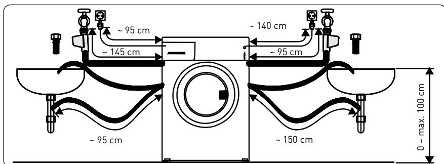
**Raccordement du tuyau de vidange**
