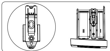
This compartment is for fabric softeners, conditioners or starch. Follow the instructions on the packaging. If the fabric softener leaves a residue after use, try diluting it or use a liquid fabric softener.
