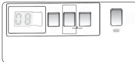
When a program is selected, the maximum spin speed is automatically selected. To adjust the spin speed between the maximum value of the selected program and no spin (- -), press the spin speed adjustment button until the desired value is displayed. If you go beyond the desired speed by mistake, keep pressing the spin speed adjustment button until the desired value is displayed again.
