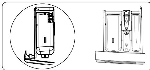
This compartment is intended for washing powder or liquid, or anti-limescale products. The graduated rule (optional) for washing liquid is provided inside the machine.(\*)
