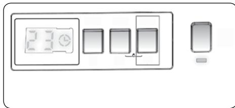
You can use this auxiliary function to delay the start of the wash cycle by 1 to 23 hours.
