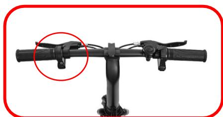
As shown in the photo, the button circled in red allows you to turn your device on and off. Push up to turn on. Then down to turn off. To turn on the front light, press the button below the battery indicator for 3 seconds.
